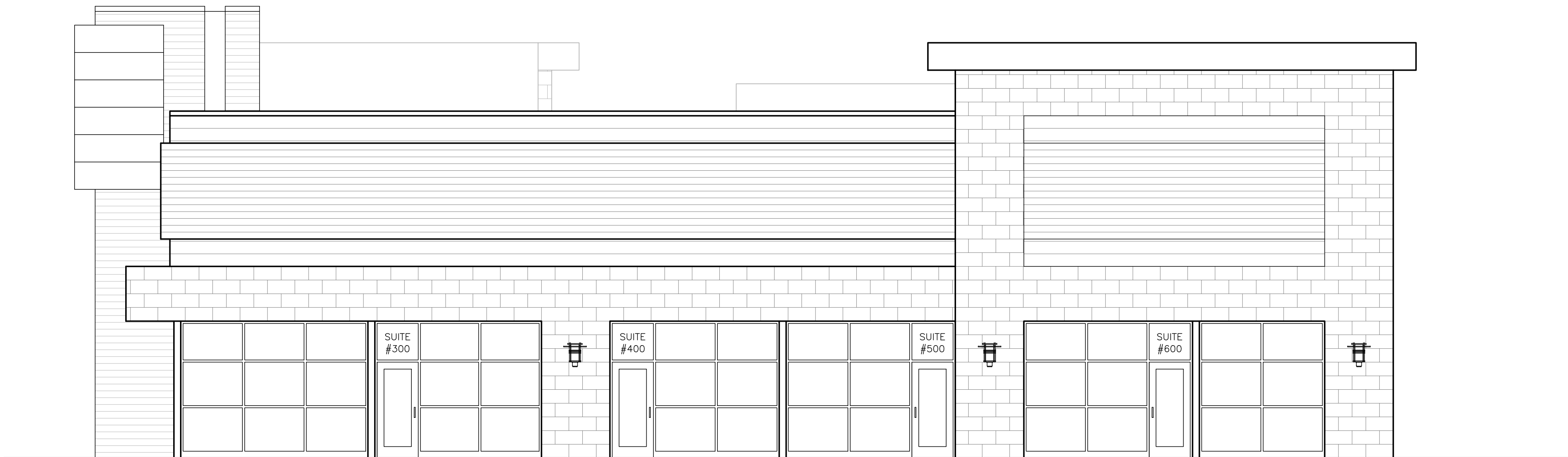
2 – SOUTH ELEVATION (MAIN FRONT) SCALE 3/16"=1'-0"
