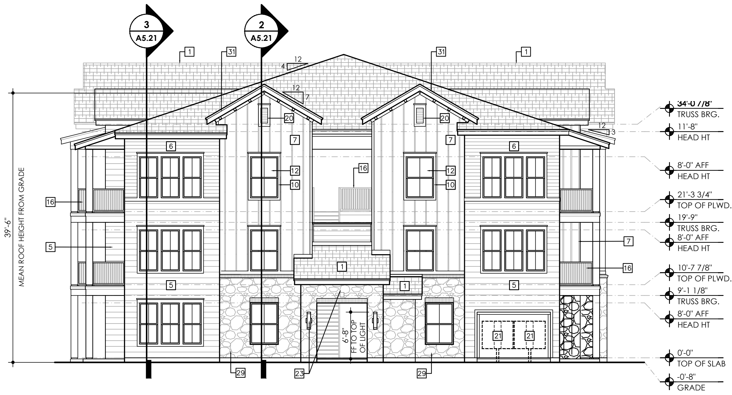
1 RIGHT ELEVATION BUILDING TYPE II
