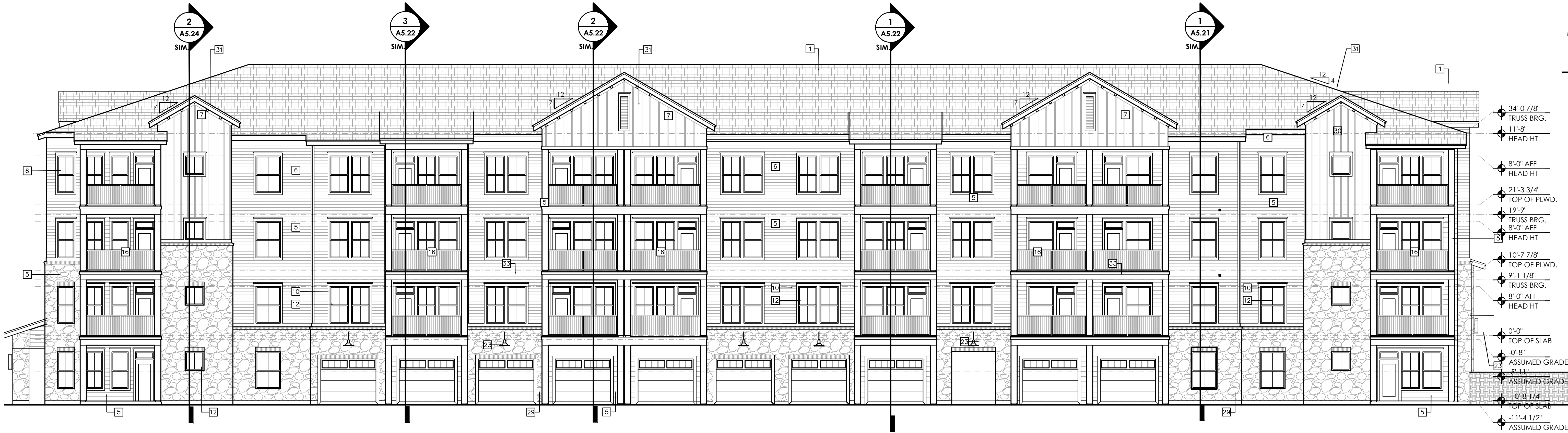
2 FRONT ELEVATION BUILDING TYPE IV SCALE: 1/8"=1'-0"
