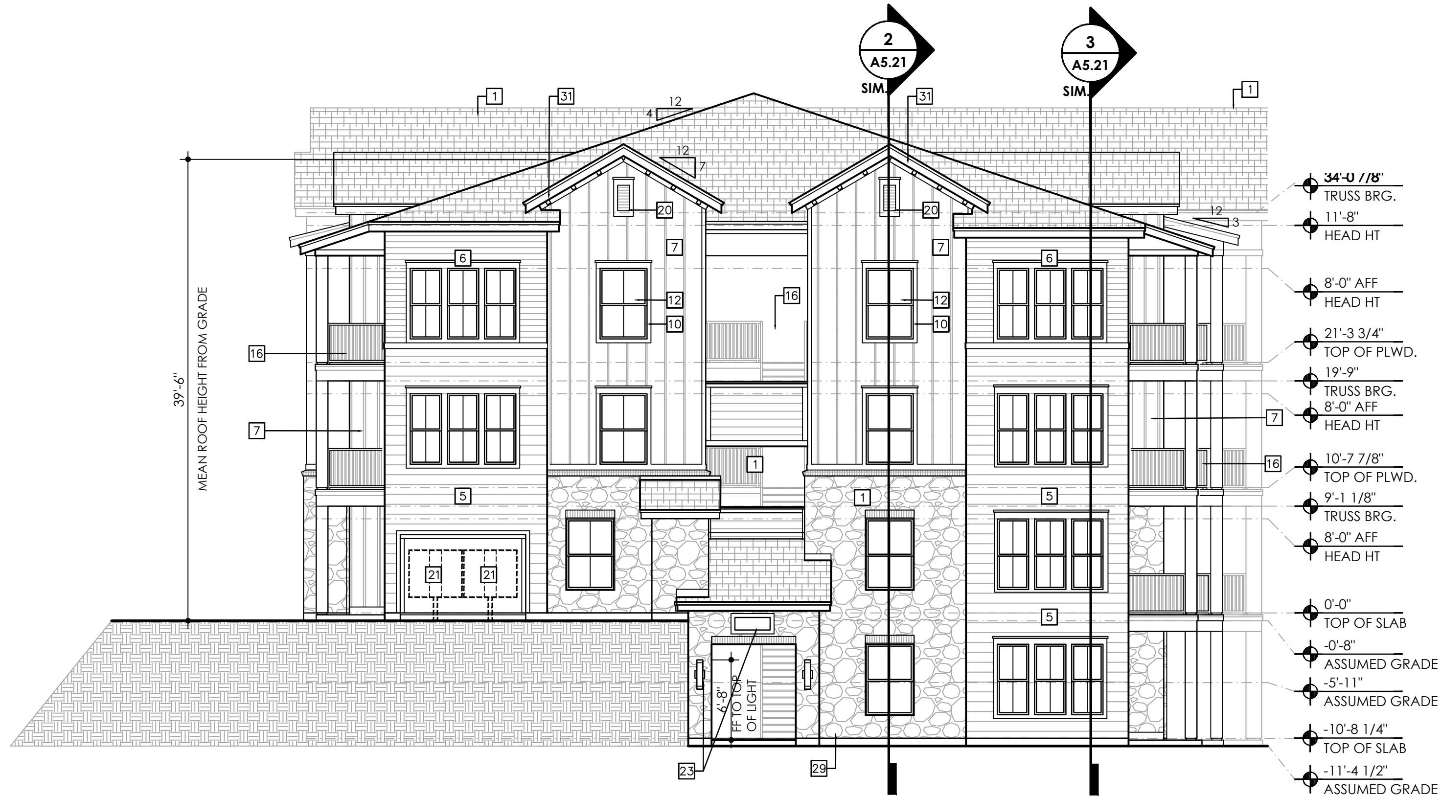
1 LEFT ELEVATION BUILDING TYPE IV
